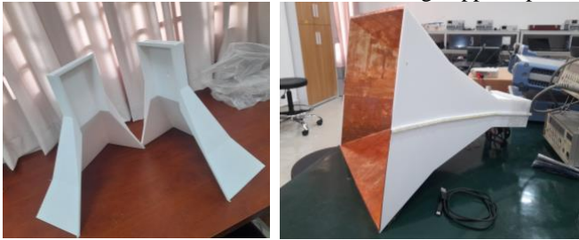
Fig. 9 Pyramidal horn antenna before (left) and after (right) materialization
