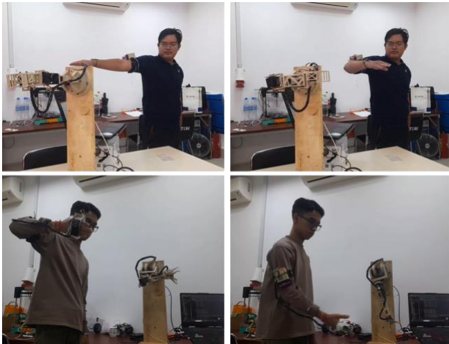
Fig. 6 Sample images illustrating complex robot movements controlled by the subject
