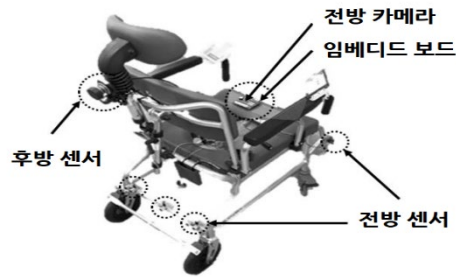
Fig. 1 Basic concept of automatic limitation of wheelchair
